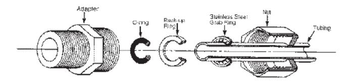
Figure 4 Typical Polypropylene Tubing Adapter Installation
