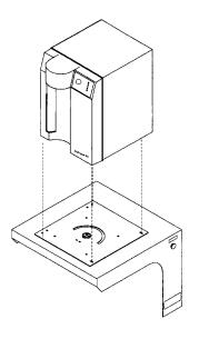
4. Install the four screws removed in step 2 through the bottom of the wall bracket and into the EASYpure RO.
